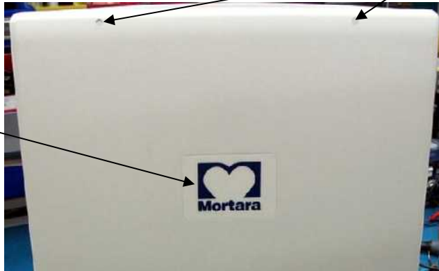
Silicon Inserts 2 plcs on rear of LCD display
